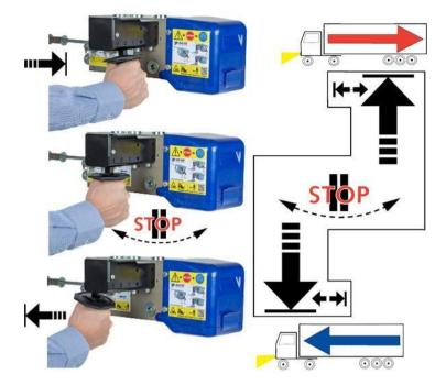
2 handle pulled out; floor will load
