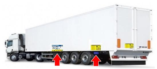
Cargo Floor drive system Cargo Floor control box **A or B control** (could be located at a different spot) (manual handle) **B or E control (switches)**
