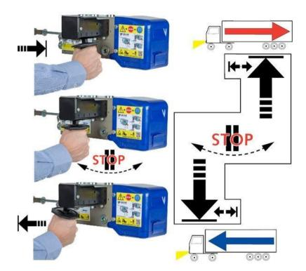
2 handle pulled out; floor will load
