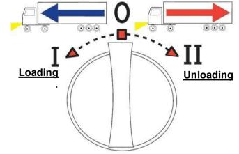
When turned left or right, it will start the floor and when released it will automatically return to the 0 position
