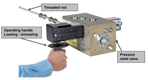
Systems fitted with A-control do <u>not</u> include any electrical operation. The system will begin to move depending on the position of the operation handle on the control valve. The handle should be positioned, before and after using the Cargo Floor, in the position stop (0) if the handle is in the position 1 or 2 the system immediately starts to move when the pump/ PTO is activated.
